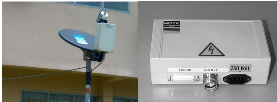
Figure 2: Outdoor and indoor components of a micro rain radar
